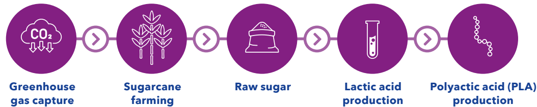
Luminy® PLA production process
